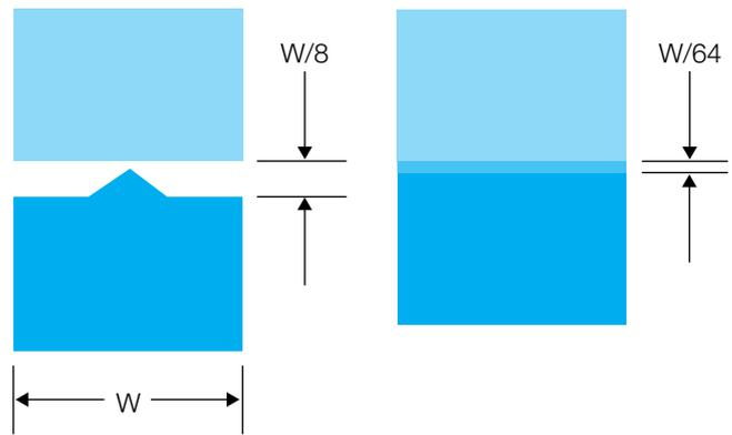
For an assembly with parts made out of two different materials, it is a general practice to design the energy director on the part with the material that has the highest melting temperature and stiffness.
